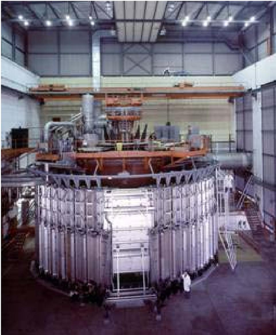
This picture shows BEBC (Big European Bubble Chamber) surrounded by the array of multiwire proportional chambers that made up the External Muon Identifier (EMI). Muons created in neutrino interactions would normally penetrate the iron return yoke of the magnet and be detected in the EMI.
