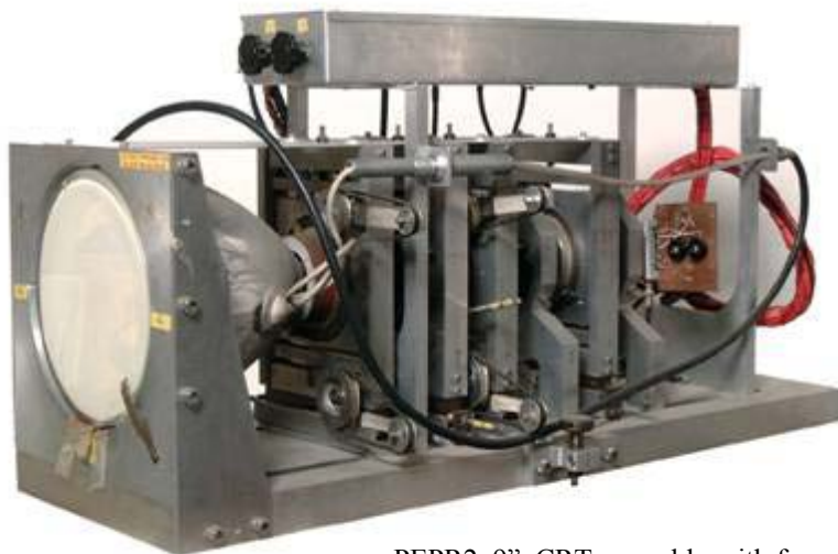
PEPR2 9" CRT assembly with focus and steering magnets
