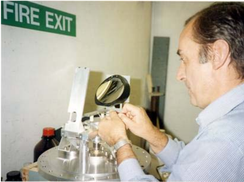
Setting up the Linford grating and light collection assembly.
