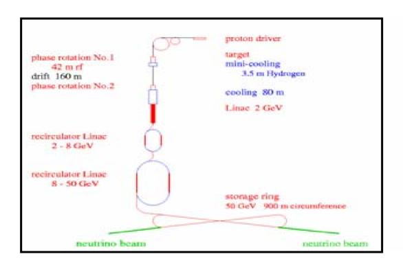
The muons produced in the pion decays have too large a spread in energy and angle to match the input of the accelerator. They must therefore be "cooled". The only feasible technique seems to be ionisation cooling. The drawing shows a potential layout for the International Muon Cooling Experiment (MICE) in which Oxford is participating. Reduction in angular spread is obtained by slowing down of the muons in liquid hydrogen, followed by acceleration in Radio Frequency cavities.
