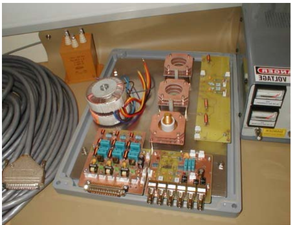
A fast power amplifier built in Oxford to power the FONT kicker
