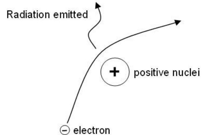
**Figure 1:** Bremsstrahlung (or 'braking') radiation is emitted when the path of a charged particle such as an electron is deviated by another charged particle. The acceleration of the electron causes it to emit a photon of light with an energy indicative of the electrons kinetic energy.
