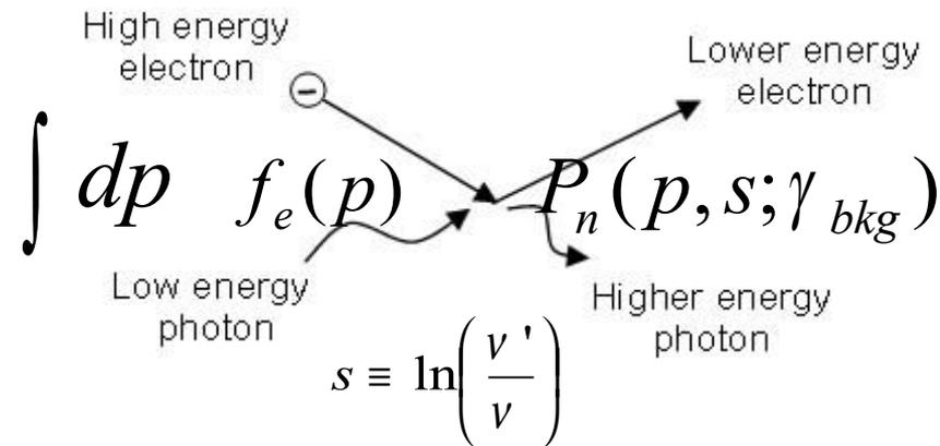
**Figure 6:** The two Compton scattering processes result in radiation being shifted to lower energies (Compton scattering) or higher energies (inverse Compton scattering). The essential factor differentiating these two processes is the kinetic energy of the electron involved.
